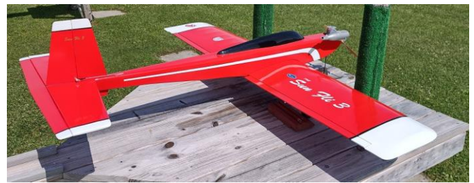
Scott Wallace's Joe Bridi Sun Fly 3 powered with an OS 61 FSR. Dope finish over silkspan/Koverall. Flies really well, as good or better than the Kaos I completed in May.
