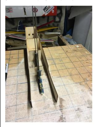
Adding 2 more formers and you are ready for putting on the bottom. I did it in 2 pieces so the back half would be flat. Again, carpenter's glue was used so you...
