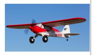
The motor is a 480-size, 960Kv BL out runner. The battery is 3S 1300-2200mAh Li-Po. Since this is a very popular plane a lot has been posted on various web sites about upgrades. There are some good suggestions there but don't plan to upgrade to a different size motor or larger battery system. The whole idea is to race a very affordable plane that is extremely easy to fly.
