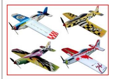
These 31" wingspan airframes are around \$70 each and come in several colors/styles; a club 4-pack is even offered at a small discount. The AGS could specify a motor/ESC/battery/prop combo and be racing. The TW hobbies motor & speed control run approx. \$50 and they recommend 3S 600 mAh Li-Po's for these racers. No, they aren't drop dead gorgeous airplanes but neither are Q-500's and something like this might be just what we need going forward for next year to renew club interest.
