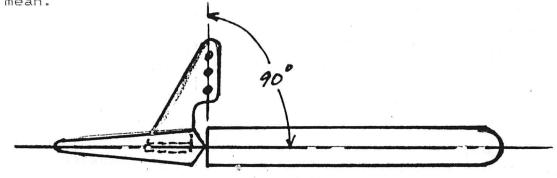
By keeping the holes in the horn at 90 degrees to the centerline of the flying surface you will get equal throw in both directions. By the way, it is easier to achieve a true 90 degree by installing the horn as I described earlier rather than mounting the horn on the surface of the tapered elevator, rudder or aileron.
