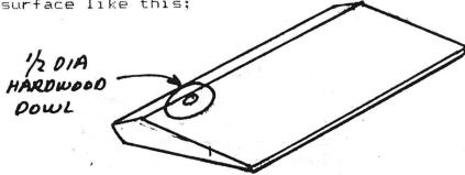
Then drill a hole at right angle to the centerline of the surface. Select a hole size that will be a tight fit on a 4-40 thread. Now after painting the plane you can screw in a 4-40 machine screw and then cut off the head. Then thread on a Goldberg 3/32" horn bracket #249. This technique provides almost infinite adjustment since all that is required is to shorten or lengthen the horn is to screw the aileron link up or down a maximum of one revolution at a time.
