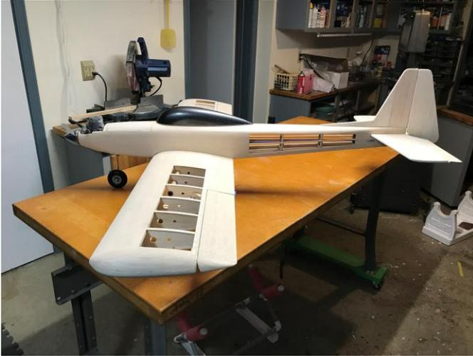
Trying to find the pieces of the fuselage was a challenge, since nothing was indicated on the plans. The cliché, “A picture is worth a thousand words.” Really doesn’t apply to a building project. With some searching, however parts were found and progress was made, thanks to carpenter’s glue and a lot of clamps. CA is an amazing glue, but I don’t like to use it when gluing any material that is not balsa. I just don’t think there is a good enough penetration into plywood, or other hard woods.
