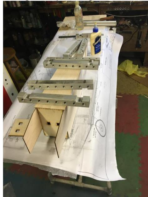
The first two formers of the Esquire form the heat of the airplane. Making them square is all important. Two squares and centerlines made this job easy. Carpenter's glue was used so you glue, step away, and wait.
