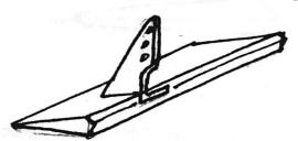
Oh, by the way, wether you install the horn with the srews or use the technique I have discussed of routing out the center of the surface don't forget to locate the horn so the holes are in line with the hinge line. Here's another sketch to illustrate what I mean.
