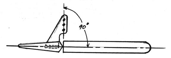
By keeping the holes in the horn at  $90^\circ$  to the center line of the flying surface you will get equal throw in both directions. By the way it is easier to acheive a true 90° by installing the horn as I described earlier rather than mounting the horn on the surface of the tapered elevator or rudder.
