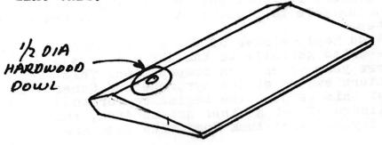
Then drill a hole at right angle to the centerline of the surface. Select a hole size that will be a tight fit on a 4-40 thread. Now after painting the plane you can screw in a 4-40 machine screw and then cut off the head. Then thread in a Goldberg 3/32 horn Bracket # 249. This technique provides almost infinite adjustment since all that is required is to shorten or lengthen the horn to screw the airleron link up or down a maximum of one revolution at a time.
